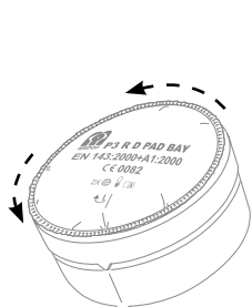
Remove the particle filter by twisting it to the left (counter-clockwise)
