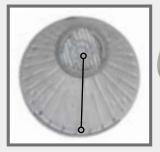
Off-centre connection for placement of the filter: provides a greater field of vision.
